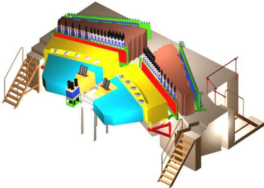
Figure 2.45: Downstream detectors installed in the DIRAC-II experimental setup. The modified Cherenkov detector can be seen in light blue. The heavy gas Cherenkov detector is represented in yellow, while the aerogel Cherenkov counter is coloured in dark blue, in the left arm.
