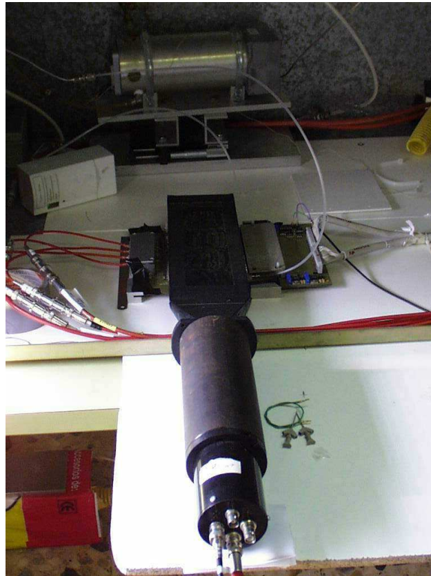
Figure 3.14: Experimental setup in Santiago laboratory. Ru^{106} source is hidden under MSGC studied plane. INa(Tl) scintillator is seen at front.
